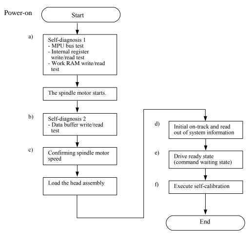
Figure 4.3 Power-on operation sequence
